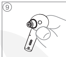
7-9. Insert the new wax guard into the opening of the sound outlet and press it gently and pull the holder straight out.
